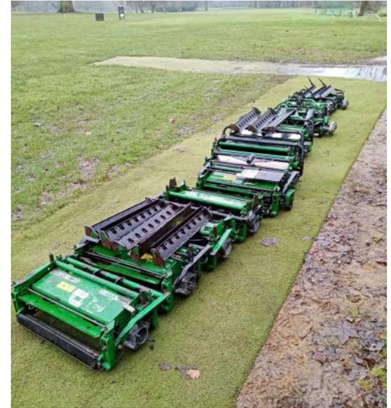
The cutting units have been stripped and are currently being sharpened, ready for the new season.
